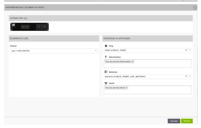
On this page, you must first choose the node to link behind this rack element. The list of nodes is filtered by node type. For example, for a UPS element you will only see UPS type nodes.
